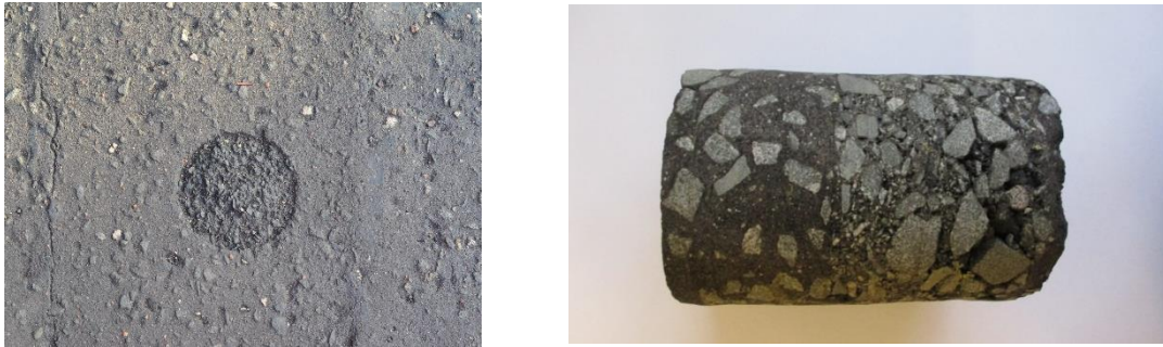
Picture 18 – Core location and sample showing surface course and binder course
